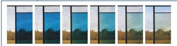
Fig. 1. Switching sequence of an electrochromic laminated glass [46].
